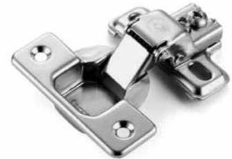
**ADJUSTMENT** (6-Way): 3mm to 5mm cup drilling distance range. +/- 2mm vertical adjustment range. -3mm horizontal adjustment range. +2.5mm depth adjustment range.
