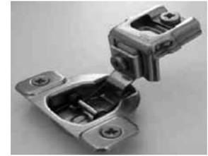
**ADJUSTMENTS** (6-Way): 3mm fixed cup drilling distance. +/- 3mm vertical adjustment range. +/- 1.5mm horizontal adjustment range. +/- 1.5mm depth eccentric cam adjustment range.
