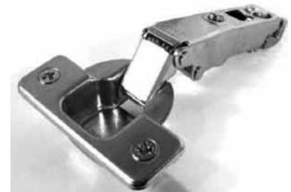
**ADJUSTMENT** (6-Way): 3mm to 5mm cup drilling distance range. -4mm / + 0.5mm horizontal adjustment range. -0.5mm / +2.5mm depth eccentric cam adjustment range. Maximum overlay 18.5mm (3/4").
