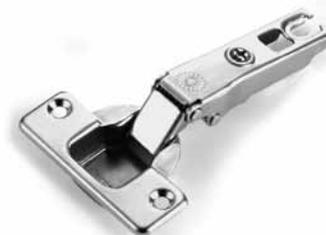
**ADJUSTMENTS (6-WAY):** 3mm to 6mm cup drilling distance range. -4mm horizontal adjustment.
